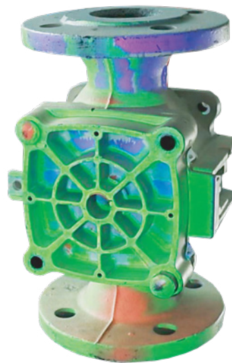
Display of the color deviation map directly on the measured object.
